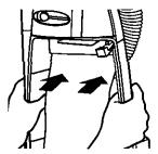
3) Install the dust bag by pressing the cardboard underneath as shown Before replacing the dust cover, make sure all edges of dust bag are completely inside the bag compartment
